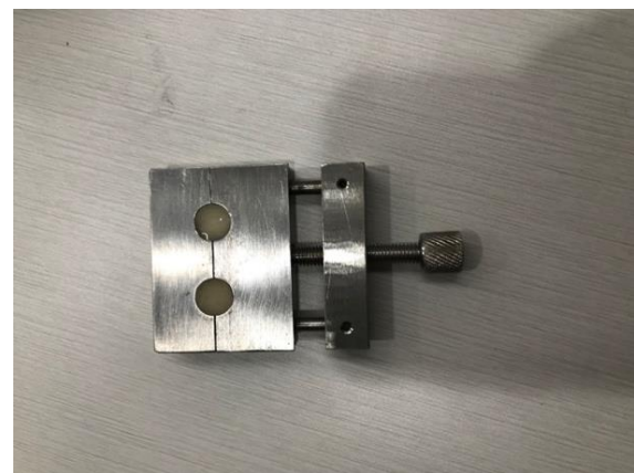
Figure 1. Sample on the stainless-steel mold
