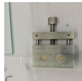
Figure 1. Resin-modified glass ionomer cement (RMGIC) sample on the stainless-steel mold
